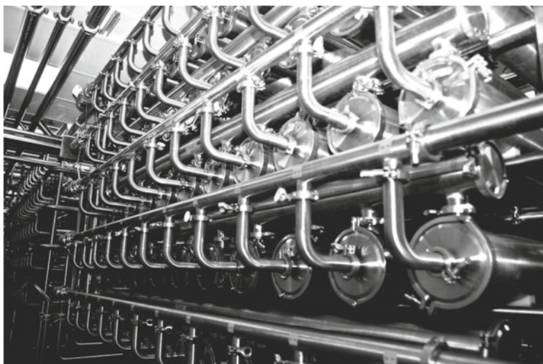
Fig. 5 Ultra filtration system (Courtesy: Milk Specialties Global)
