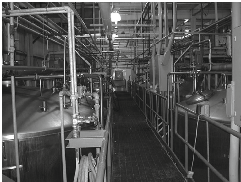
Fig. 2 Bank of hydrolysis reactors (Courtesy: Kerry Biosciences)
