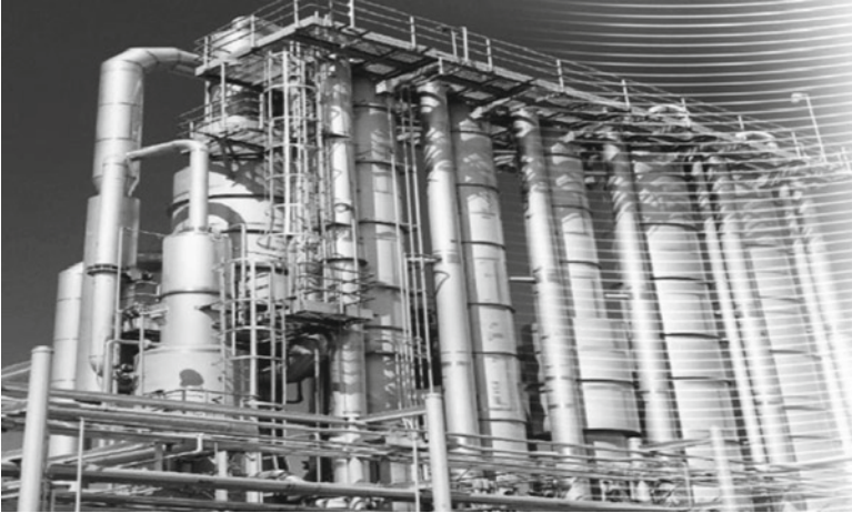
Fig. 6 Falling film evaporator (Courtesy: Niro Inc.)
