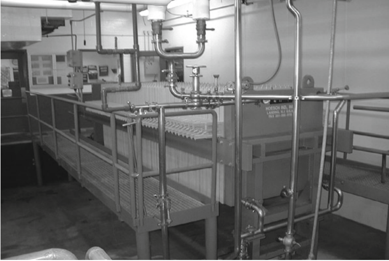
Fig. 3 Plate and frame filter press (Courtesy: Kerry Biosciences)
